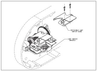
Figure 12A. Rotatable Limit Switches, Models J, JJ, L, LL, R, RR, & RRS
