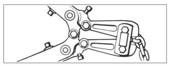
Figure 16. Cutting Chain with a Bolt Cutter
