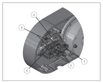
Figure 12. Limit Switches, Models J, JJ, L, LL, R, RR, & RRS
