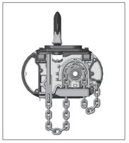
Figure 3. Attaching Load Chain Double Reeved Models
