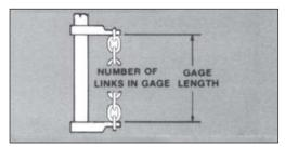
Figure 9. Gaging Load Chain Wear
