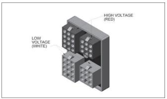
Figure 5. Voltage Change Board
