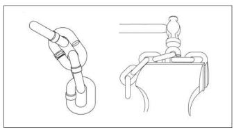
Figure 15. Cutting Chain by Nicking
