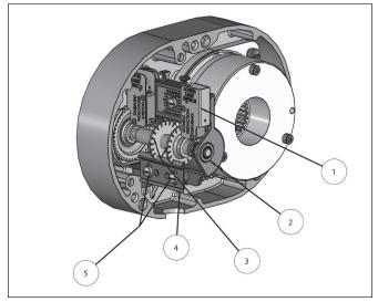
Figure 11. Limit Switches, Models B, C & F
